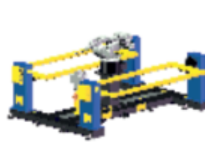
Head and tail welding station
